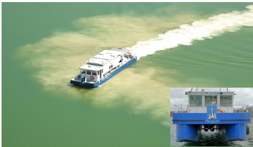
Fig. 4 In-lake-neutralization in a Lusatian mining lake by means of the “Barbara” vessel. Inset: input system between the vessel’s hulls. Source: LUG/LMBV.
